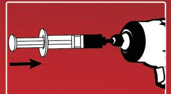
D. Inject the grease into the anvil grease hole, to complete.
