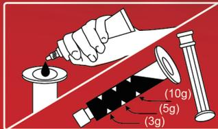
B. Squeeze the grease into syringe to the quantity mark is for NC-6266H(10g), then set the plunger. (Please do not open the syringe cover at this moment.)
