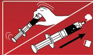
C. Holding the front end of syringe, shake the syringe until the grease is in front end of syringe, open the cover, push the plunger for expanding the air in the tube.
