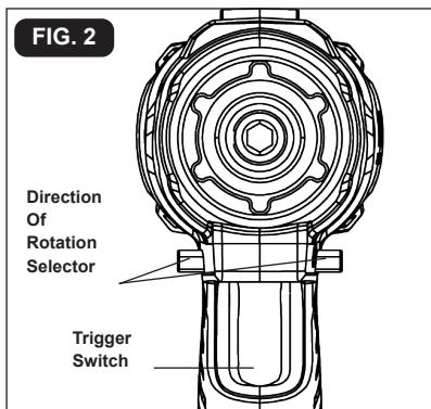
1. To turn the impact driver on, depress the trigger switch.
