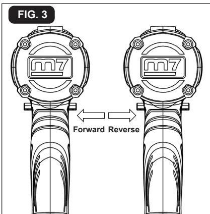
The direction of rotation is reversible and is controlled by a selector located above the trigger switch. With the impact driver held in normal operating position: position the direction-of-rotation selector to the left of the tool for forward rotation; position the direction-of-rotation selector to the right of the tool for reverse rotation. Setting the switch in the OFF (center-lock) position helps to reduce the possibility of accidental starting when not in use.
