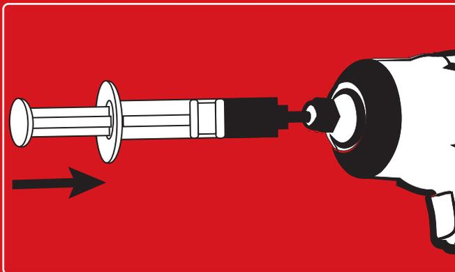
**D.** Inject the grease into the anvil grease hole, to complete.
