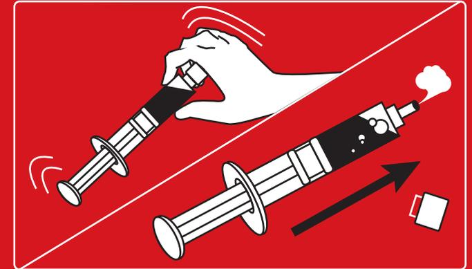
**C.** Holding the front end of syringe, shake the syringe until the grease is in front end of syringe, open the cover, push the plunger for exhansing the air in the tube.
