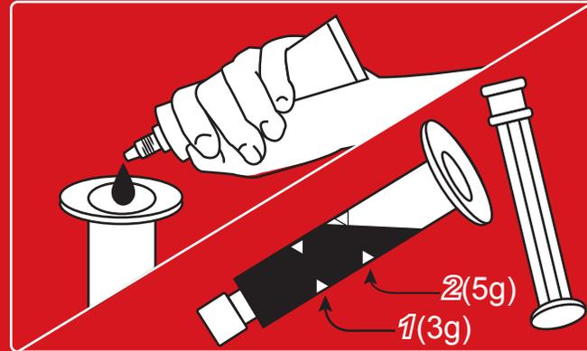
**B.** Squeeze the grease into syringe to the quantity mark ① is for NC-4650(3g). ② is for NC-4233 & NC-4255(5g), then set the plunger. (Please do not open the syringe cover at this moment.)
