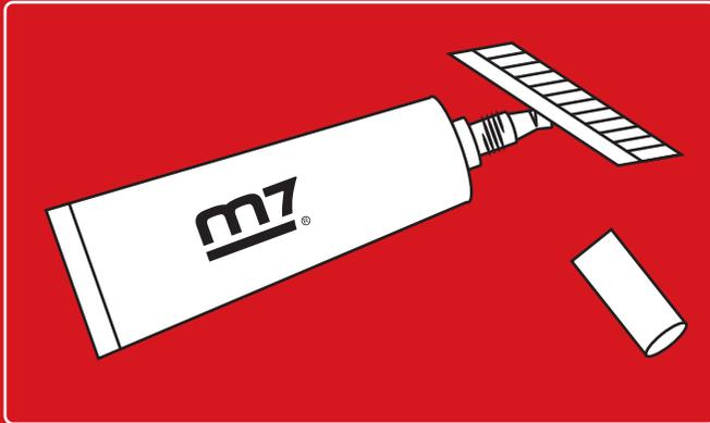
**A.** Take off the tube cap, using a knife to cut the front end of tube.
